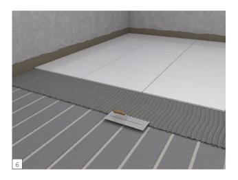
Ceramic tiles with a minimum size of  $10 \times 10$  cm can be laid on this surface. The wedi PreLine can be tiled directly after reinforcement without further pretreatment. Laminate or complete parquet must be laid as a floating floor.
